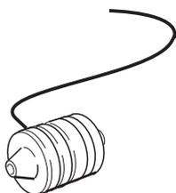
The flow cell has two cylindrical titanium electrodes positioned in the flow path of the cell. An alternating voltage is applied between the electrodes and the resulting current is measured and used to calculate the conductivity of the eluent. The monitor controls the AC frequency and increases it with increasing conductivity between 50 Hz and 50 kHz giving maximum linearity and true conductivity values.
