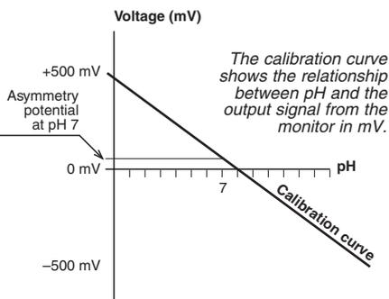
A new electrode typically has a slope of 95 - 102% and an asymmetry potential within  $\pm 30$  mV. As the electrode ages, the slope decreases and the asymmetry potential increases.
