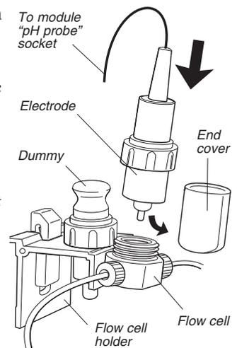
*Note: If the electrode is not fully inserted, the system will leak and a dead volume will occur in the holder.*
