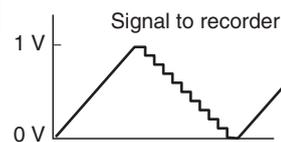
The test will ramp the signal on each channel up to 1 V and then decrease the signal in 10% steps back to 0 V. The test is run continuously. Compare the diagram of the chart recorder with the figure.
