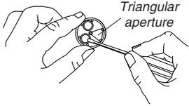
**Note:** Filters are sensitive optical components. Never touch the optical surfaces or expose them to temperatures above 60 °C. Clean them with dry lens cleaning tissue and store them, when not in use, in the box in which they were supplied. Heavy contamination may be removed by using a lens tissue dipped in ethanol.
