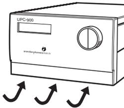
The module should be located in a place of low temperature variations, away from heat sources, draughts and direct sunlight.
