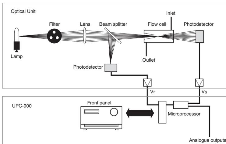
The reference signal comes from the same point in the lamp as the signal measuring the sample, thus assuring a stable baseline by eliminating the effects of variations in lamp intensity.
