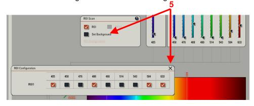
**PS**: Once the ROI background box is unchecked, the power in the laser lines will go back at their original values established for the ROI scan.
