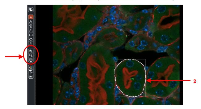
**3. a)** Activate the ROI background button, and **b)** reduce the power laser(s) until the region outside the ROI is completely black.
